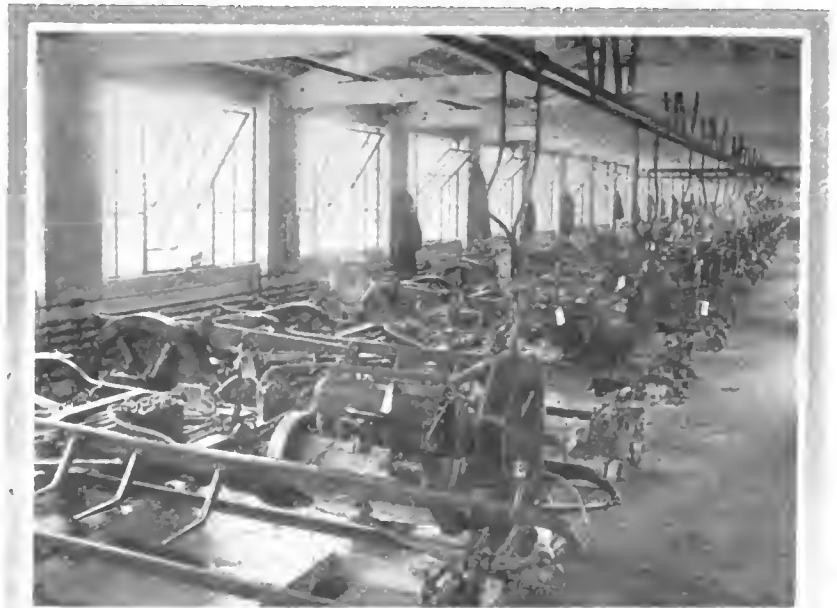
Studebaker chassis testing room showing six-cylinder cars undergoing their first trial under load. There is room for nineteen cars at one time in the 300-foot building. Each radiator connects to the circulating water mains which communicate with a tank. The gasoline is also supplied to each chassis from a main pipe
